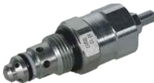
The **main relief valve** is fitted in a SAE08 (3/4-16UNF) cavity. It is designed to improve pressure setting, stability whilst avoiding the noisy operation typical of lower cost alternatives.
