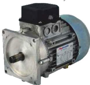
**B14 IEC and Nema standard AC motors:** commodity motors easily available in every market from 0,18 to 7,5 kW, single or three phase. These motors are normally procured and mounted by the customer himself. Hydronit provides adaptor flanges and two piece coupling for frame sizes: 63, 71, 80, 90, 100 and 112 (IEC) + 56C and 184TC (Nema).
