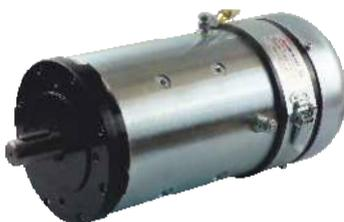
**Frame 151 DC motors:** heavy duty motors, with fan cooling, thermal protector and running time of 16 min or over. Power from 2,5kW up to 4kW, 12 or 24VDC.
