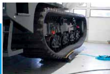
Lifting for track maintenance - Construction Machinery -
