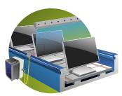
The timer was set to the "interval" setting when detecting the flat panel displays. The sensor was mounted 1" (25mm) prior to the Super Ion Air Knife blowoff station. When it detected the flat panel, it turned the air on immediately and started the 10 second timing sequence for closing the valve (shutting the air off). In the event the conveyor stopped, the air would no longer cycle on again until the next flat panel was detected.
