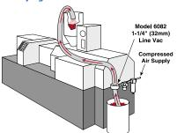
**The Problem:** Injection molding machines transform plastic pellets into various plastic products. The pellets are gravity fed from a hopper on top of the machine. The "bucket and ladder" method of replenishing the hopper was inefficient and expensive.
