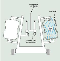
**The Problem:** Automobile fuel tanks are blow molded, then clamped to a fixture to prevent distortion during the cooling cycle. The cooling time of over 3 minutes required for each tank created a bottleneck in the production process.
