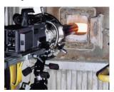
Special high temperature vortex tubes keep a boroscope lens cool while inserted into a 1200°F (650°C) boiler porthole.
