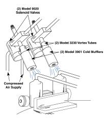
**The Problem:** Air conditioner parts assembled on an automatic brazing machine must be cooled to handling temperature prior to removal. The machine was capable of brazing up to four hundred pieces per hour. However, the time required for the parts to cool severely limited the production rate. Water cooling was unacceptable from the standpoint of both housekeeping and part contamination.
