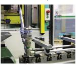
A pair of medium vortex tubes cool a solenoid coil after a welding operation.
